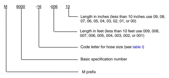
PIN example: M6000-H-00610 describes a 1-inch inside diameter hose that is 6 feet 10 inches long.
